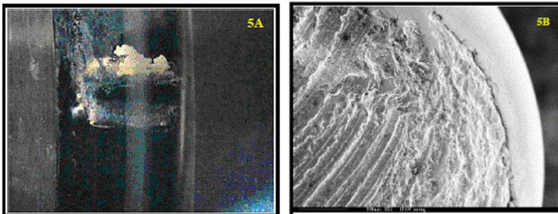
**Figure 5.**Damage to bearing due to Corrosive wear (5A) and Surface Fatigue (5B).
