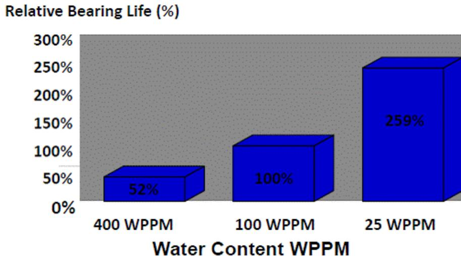
**Figure 7.**Relative Bearing Life vs. Water Content
