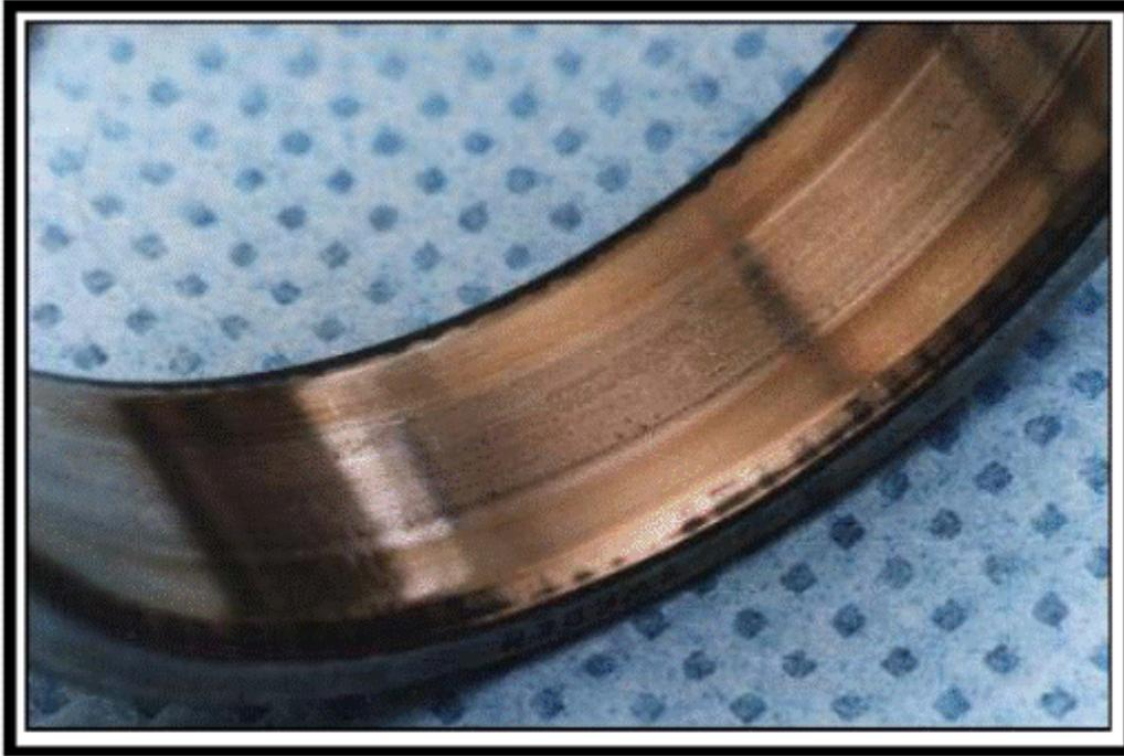
**Figure 4.**Damage to bearings due to Abrasive wear
