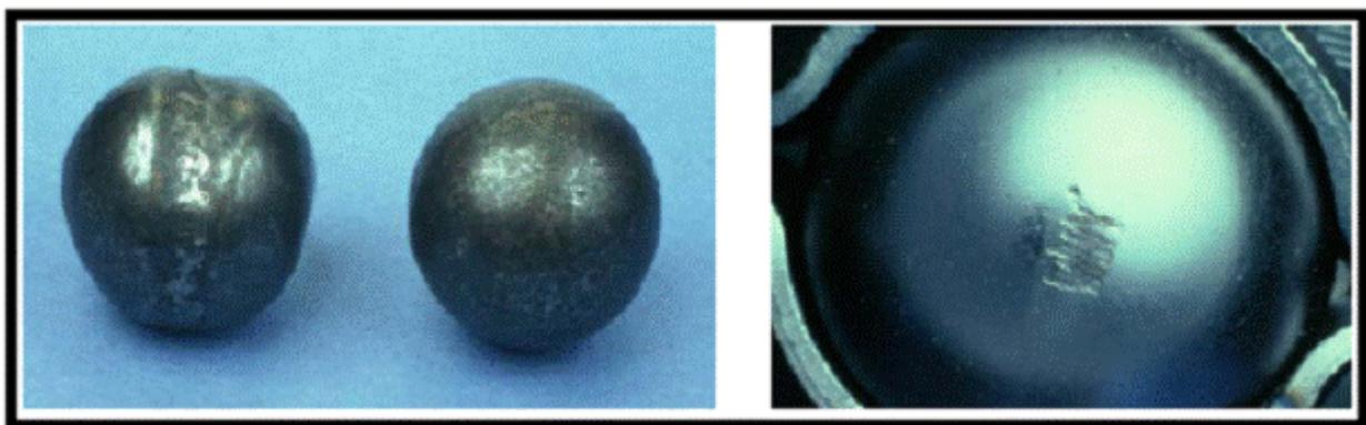
**Figure 3.**Damage to bearings due to particulate within lubricating oil.
