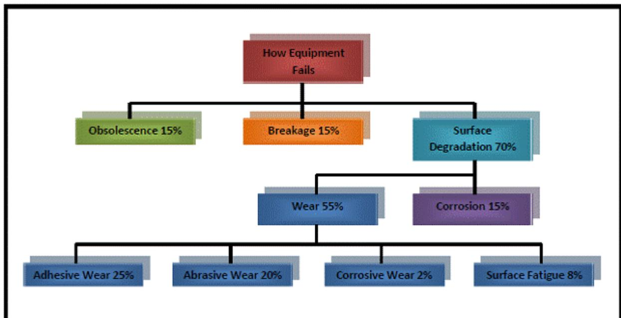
Figure 1. How Equipment Fails Flow Chart, Rabinowicz, 1981.
