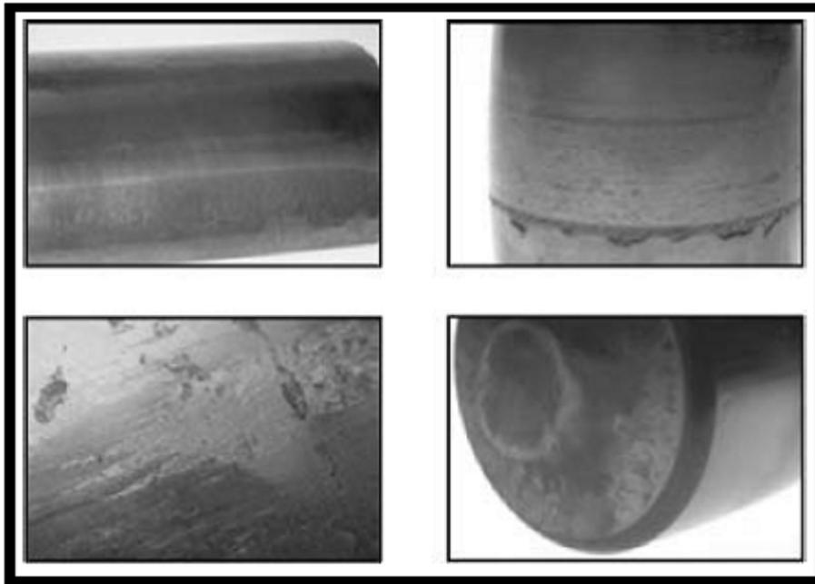
**Figure 2.**Damage to bearings due to adhesive wear.
